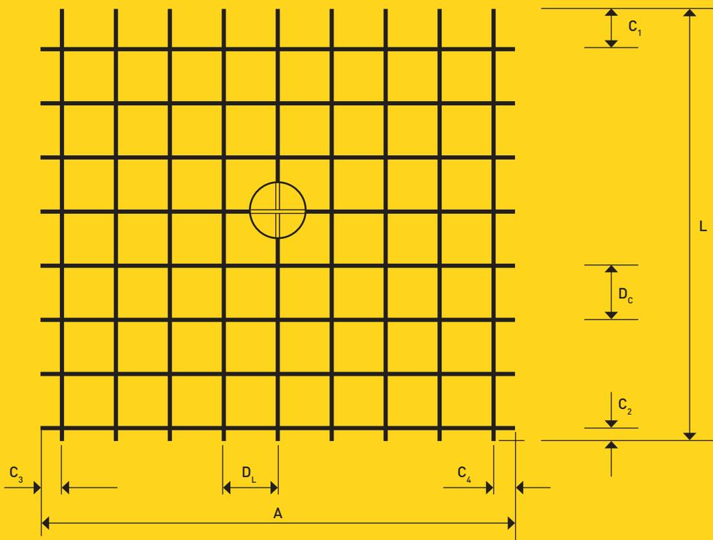
Figure 1: Geometric Characteristic of Welded Fabric.
