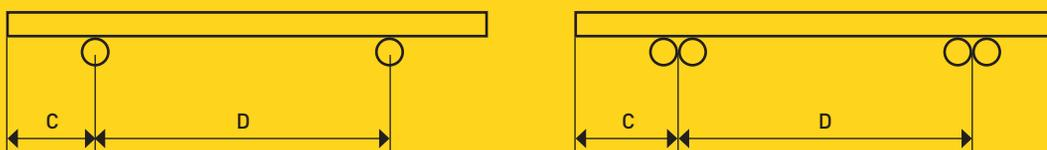
Figure 2: Pitch of the Wires (D) and Overhangs of the Wires (C).
